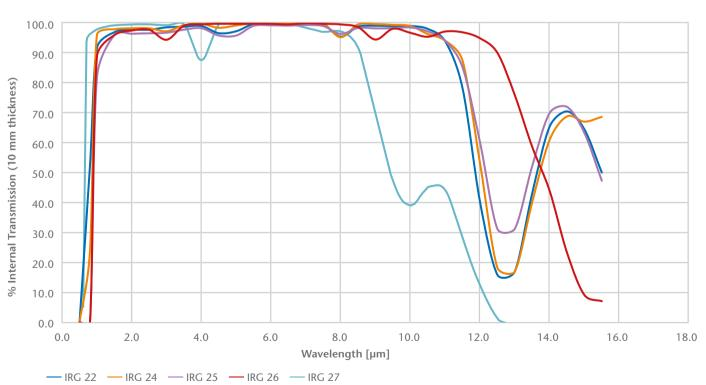
Internal Transmission of Infrared Glass IRG 22, IRG 24, IRG 25, IRG 26, IRG 27 with Thickness 10.0 mm (Typical Values)
